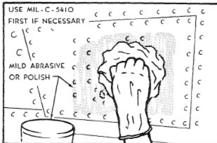
Figure 6-12. Polishing and Brightening Alclad Surfaces
