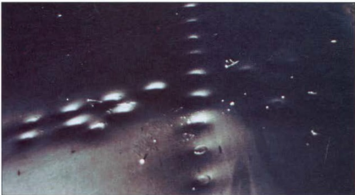
Figure 4-12. Skin Bulging Around Fasteners
