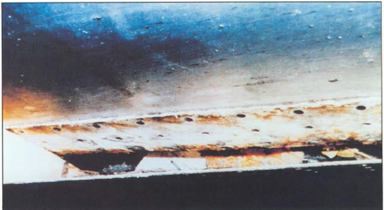
Figure 5-15. Severely Corroded Lap Joint
